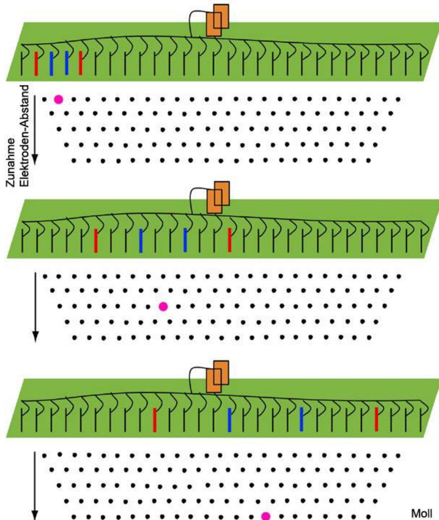
In **2D ground resistivity measurements**, the four-point electrodes are gradually shifted horizontally and their spacing is increased. This produces a dataset that captures both horizontal and vertical variations of the subsurface. Using forward-modeling software, a two-dimensional resistivity profile of the subsurface is calculated.
