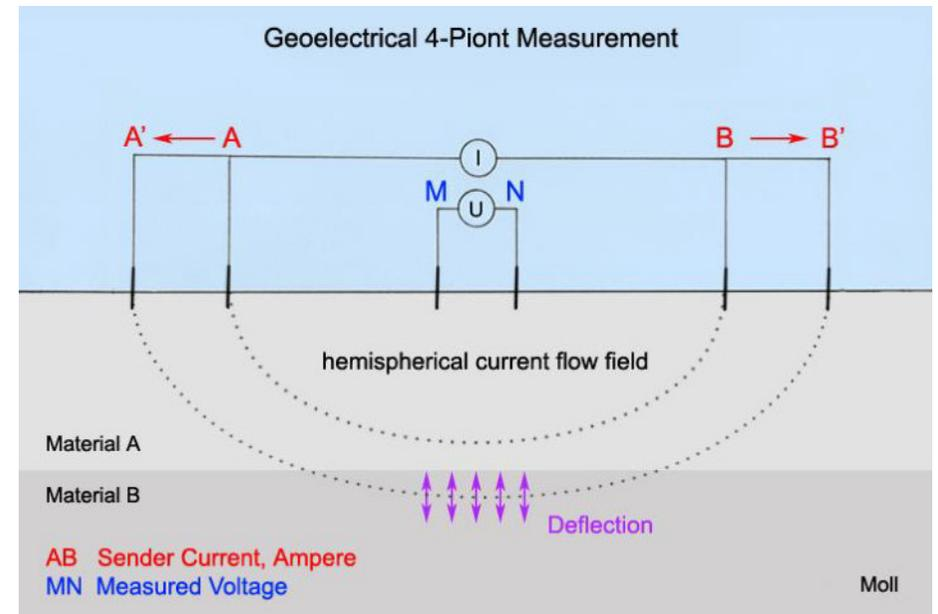
Deformation of Geo-Electrical Current Fields Depending on Changes in Ground Conductivity:<sup>1</sup>
