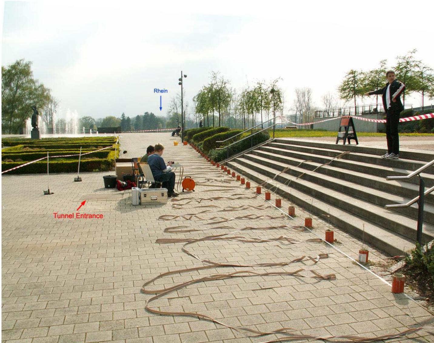
Measurement\_01: Electrode Cable Setup (Moll)
